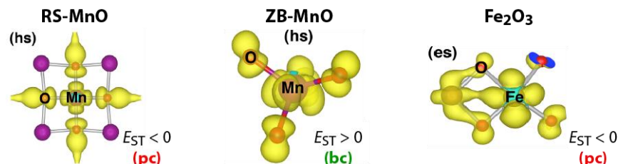
Figure 2: Wave-functions of the self-trapped (small-polaron) state; sign of E_{ST} indicates band or polaron conduction (bc or pc).
