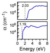
Density of states (DOS) and absorption spectrum, shown for  $Cu_2O$  and CuO.
